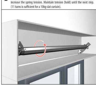
Turn the tube approximately 10 turns in the downward direction, to
