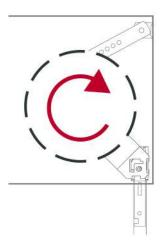
To INCREASE tension: Rotate the curtain in an downward direction inside the box.
