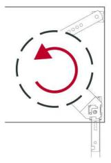
To **REDUCE** tension: Rotate the curtain in an upward direction inside the box.
