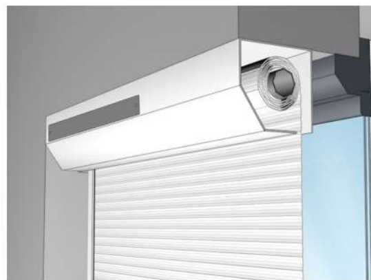
Recess fit A: Outward roller
