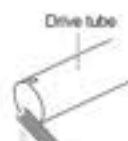
Step 2: Ensure tube edge is clean and burr-free.
