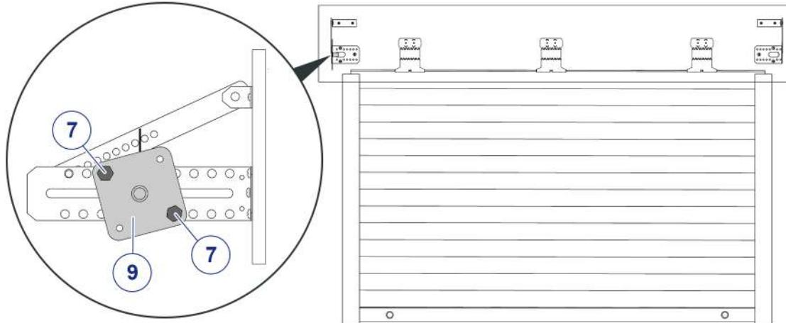
Raise the first slat and attachment clips, then position the tube.
