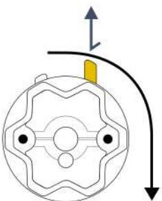
If the motor is running in this direction, press and release the yellow button
