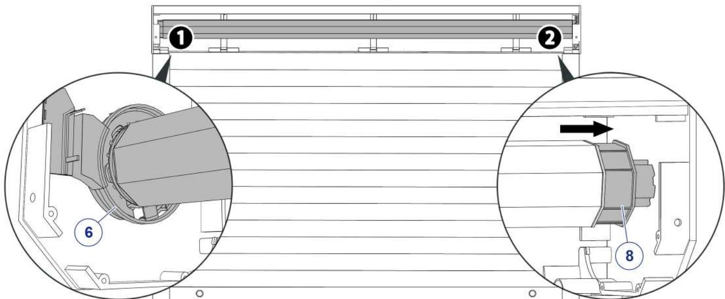
**16** Attach the tube end to the axle.
