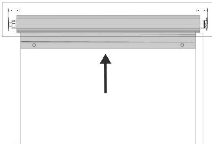
**e** Lower the shutter with the control, it should stop near the bottom. If the motor continues after it's reached the bottom, press **STOP** and make a few turns to the **-** on the lower adjustment screw.
